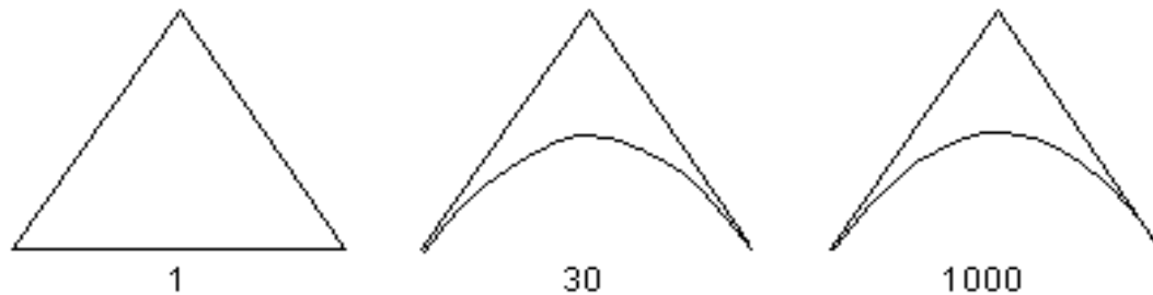
Figure: Jacobian Ratios for Triangles
