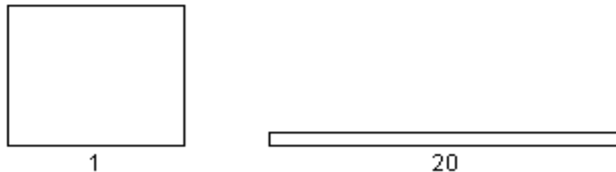
Figure: Aspect Ratios for Quadrilaterals
