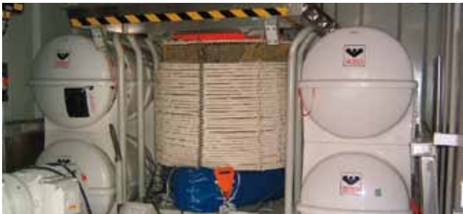
Liferafts are an integrated part of the system and safely stored inside the blast proof container
