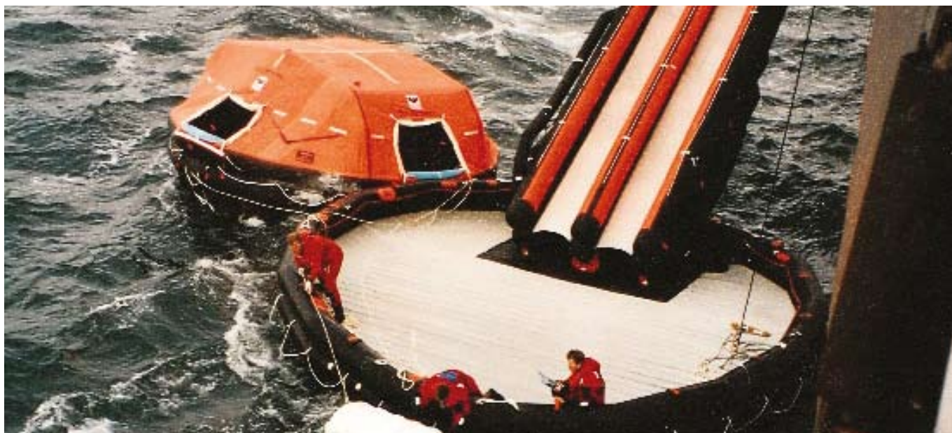
The platform can receive evacuees before the liferafts are fully inflated, saving valuable time.
