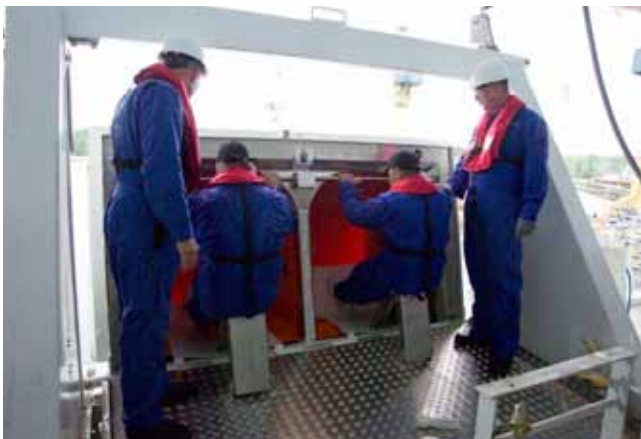
The dual chute system is easy to operate and requires few trained crew members.
