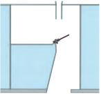
Open joint with drainage
