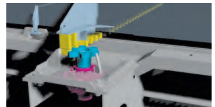
A rack and pinion drive
