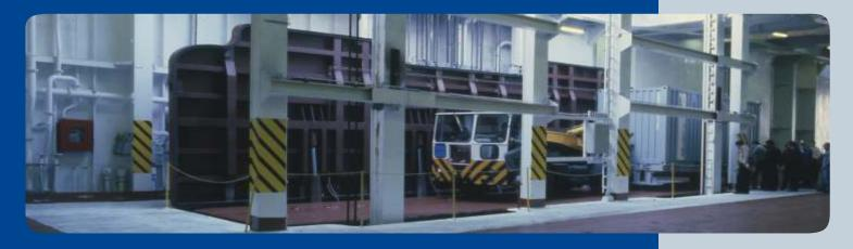
avalimpianti elevators provide solution for transferring provisions, vehicles, pallets and forklifts between different deck levels when longitudinal spaces are limited.
