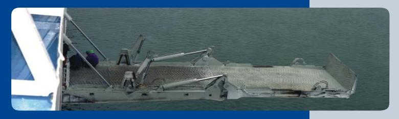
avalimpianti Tecnimpianti side ramps are designed for loading and unloading vehicles and trucks when high degree of cargo access flexibility is requested. The correspondence to any ship dimensions and to the range of quay heights assures high operational efficiency.
