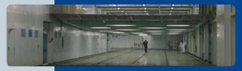
avalimpianti Tecnimpianti car decks are designed for the vertical stowage when not in use or, alternatively, for quick vertical adjustment, permitting the loading of cars and the arrangement of wheeled cargos of variable height.
