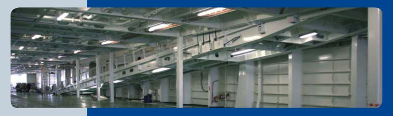
avalimpianti Tecnimpianti hoistable & tiltable ramps assure a great flexibility of vehicles transiting between two different deck levels. In addiction, ramps may be raised or lowered while carrying trailers and cars, according to the specific load requirements.
