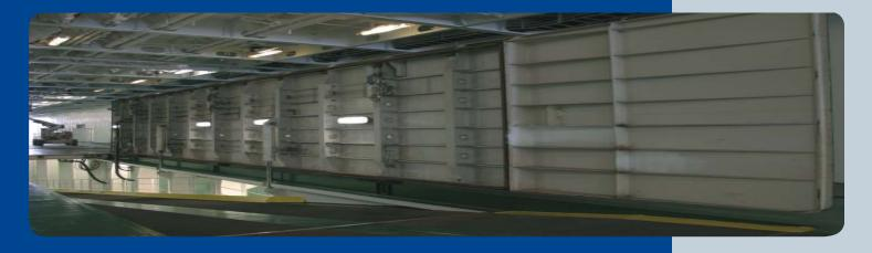
avalimpianti Tecnimpianti internal facilities for RoRo vessels include covers and doors available in different arrangements to meet customer's applications.
