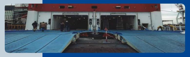
argo access facility on RoRo vessels includes stern ramps for loading and unloading trailers, cars and for passengers boarding.
