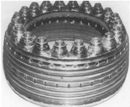
JT9D annular combustor.
