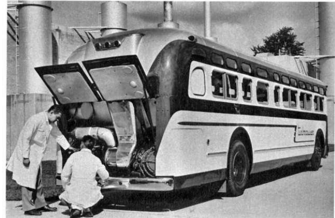
Turbocruiser coach is a conventional General Motors bus equipped with a GT-300 gas turbine and special instruments.
